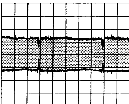
②6 R298 CN102 Pin ③ PB RF (PB) VOLT/DIV : 50mV TIME/DIV : 2mS
