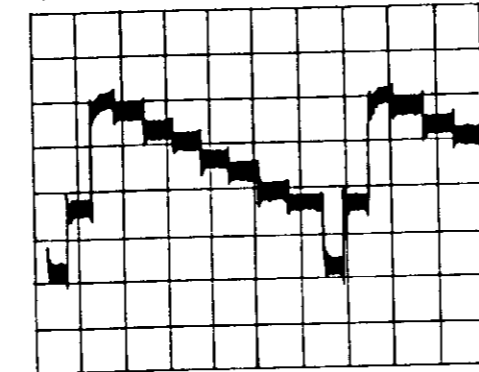
③ IC101 Pin ⑦ (PB) VOLT/DIV : 200mV TIME/DIV : 10 μ S
